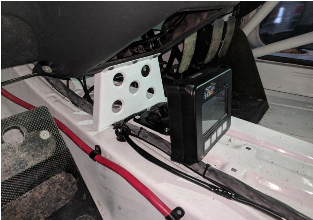
Figure 2. The WRC tracking unit mounted onto the 25mm rubber ball mount and connected through the RallySafe connector
