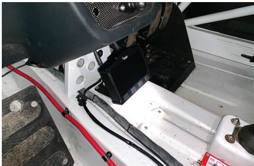
Figure 2. The WRC tracking unit mounted onto the 25mm rubber ball mount and connected through the RallySafe connector.
